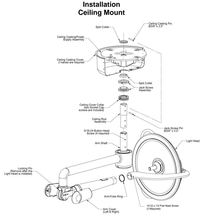
Figure 5: Shown, sub-assemblies for a Solo, ceiling mount. The same installation applies for the Duo & Trio. Note: Do not remove locking pin until light head is installed on arm.
