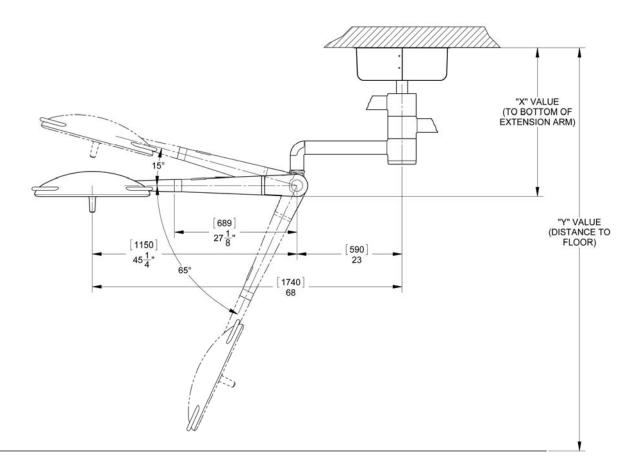
Figure 4: Ceiling Rod Calculation Trio Mount
