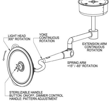
Figure 14: Head and Arm Movement (Solo light shown)
