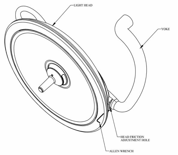
Figure 17: Light Head Adjustment
