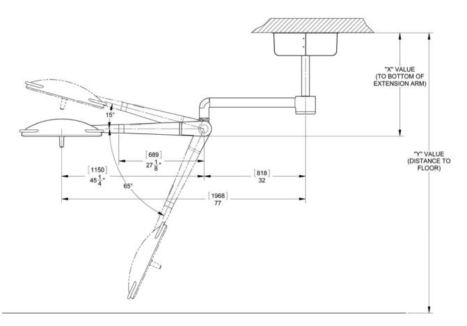
Figure 2: Ceiling Rod Calculation Solo Mount
