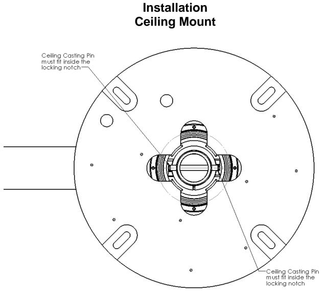
Figure 11: Ceiling & Shaft dowel pin locking.
