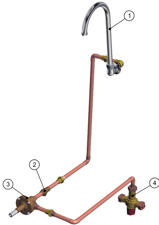
Fig. 10: Manual knee operated sink plumbing
