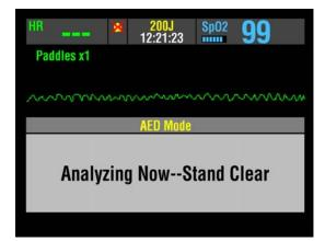
When the ECG waveform is set to ON in the setup options (refer to Section 8), the ECG appears with all of the AED messages and prompts, as shown in the screen to the left.
