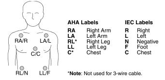
Figure 3-3 Electrode Placement for ECG monitoring
