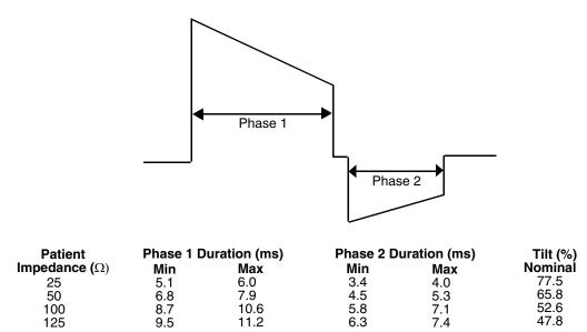
Note: Tilt is the amount of slope in waveform, expressed as the amount the current or voltage drops before truncation. A 100% tilt waveform would be termed nontruncated.
