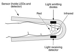
Figure 3-4 How a Pulse Oximeter Works
