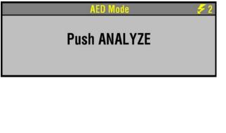
If the motion is detected during the ECG analysis, you will see and hear MOTION DETECTED, STOP MOTION followed by a warning tone. Analysis is inhibited up to 10 seconds. After 10 seconds, even if motion is still present, the analysis proceeds to completion. Refer to Table 4-1 for possible motion causes and suggested solutions.
