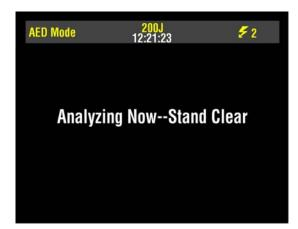
When the ECG waveform is set to OFF in the setup options, the messages and prompts fill the screen as shown in the screen to the left.
