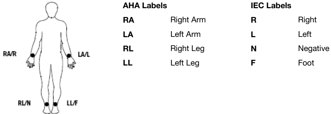
Figure 18 Limb Lead Electrode Placement for 12-Lead ECG
