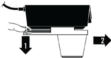
Figure 41 Removing a Pediatric Paddle
