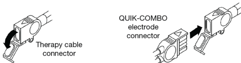
Figure 36 Connect QUIK-COMBO Electrodes to Therapy Cable
