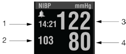
Figure 26 NIBP Measurements and Timer
