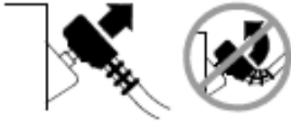
Figure 5-7 Disconnecting Defibrillation Cable from Test Post
