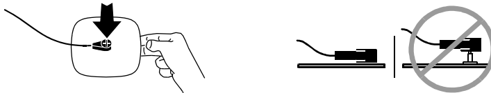
Figure 5-4 Connecting FAST-PATCH Electrodes to Defibrillation Cable
